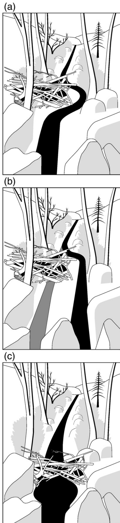
Fig. 5. Channel alterations by woody debris accumulation, as observed in the study area.
